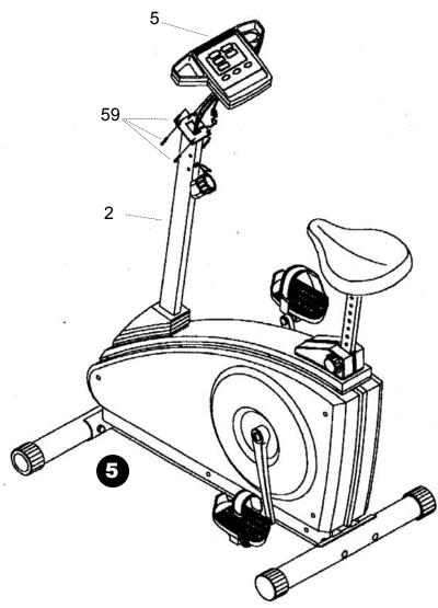
**5.** Connect the computer cable at the top of the console tube (2) to the console (5). Both computer cable connections have white ends. Feed the pulse wires from the console (5) down into the console tube (2) and out the front hole in the handlebar area. Attach the console tube (2) to the console (5) with the screws (59) provided and already attached to the back of the console (5).
